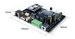
Up2Stream AMP2.0 is a WiFi and Bluetooth 5.0 amplifier board that can be applied into your regular audio system to make them wireless enabled. With this all-in-one solution amplifier board, on the 4STREAM application, you can play the same music to each room in sync or play different music to different rooms.
