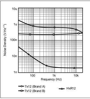
**Output noise density**. Even though the internal reference has no filtering at all, noise is as low as the Johnson noise of a  $250\Omega$  resistor.
