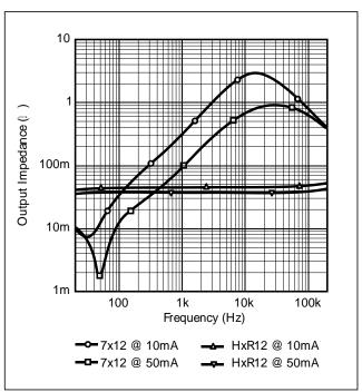
Output impedance at two load currents.
