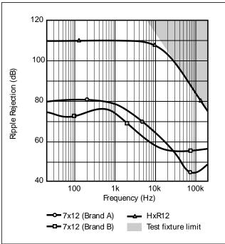
**Ripple Rejection.** HF ripple rejection is dominated entirely by magnetic coupling in the test fixture.
