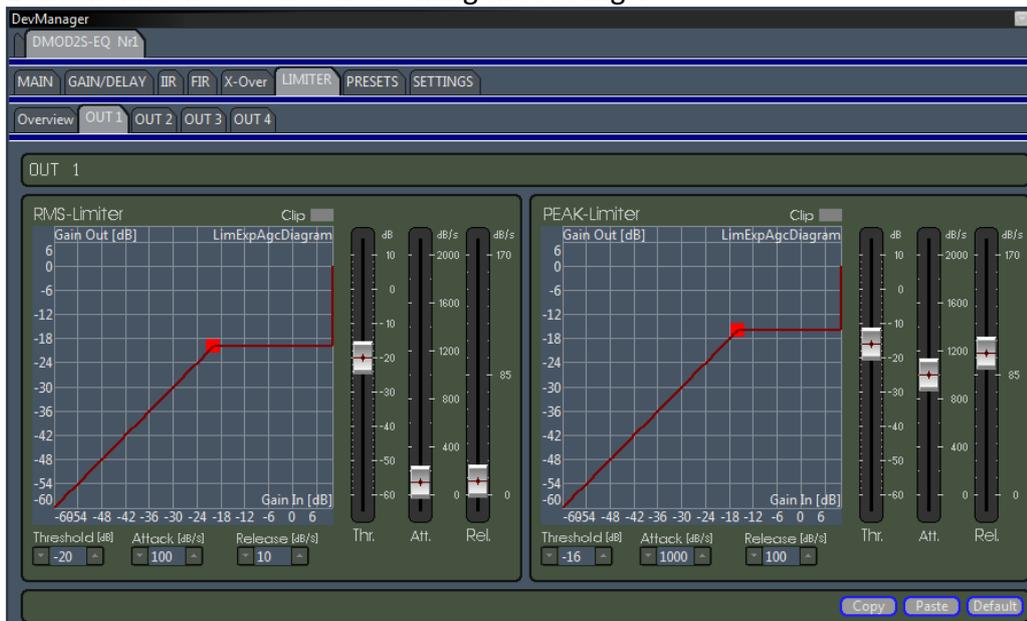
The screenshot shows the sub-tab for OUT 1. It displays two limiter settings: RMS-Limiter and PEAK-Limiter. Each limiter has a graph showing Gain Out [dB] vs Gain In [dB]. The RMS-Limiter graph shows a threshold at -20 dB. The PEAK-Limiter graph shows a threshold at -16 dB. Below the graphs are sliders for Threshold [dB], Attack [dB/s], and Release [dB/s]. There are also buttons for Copy, Paste, and Default.
