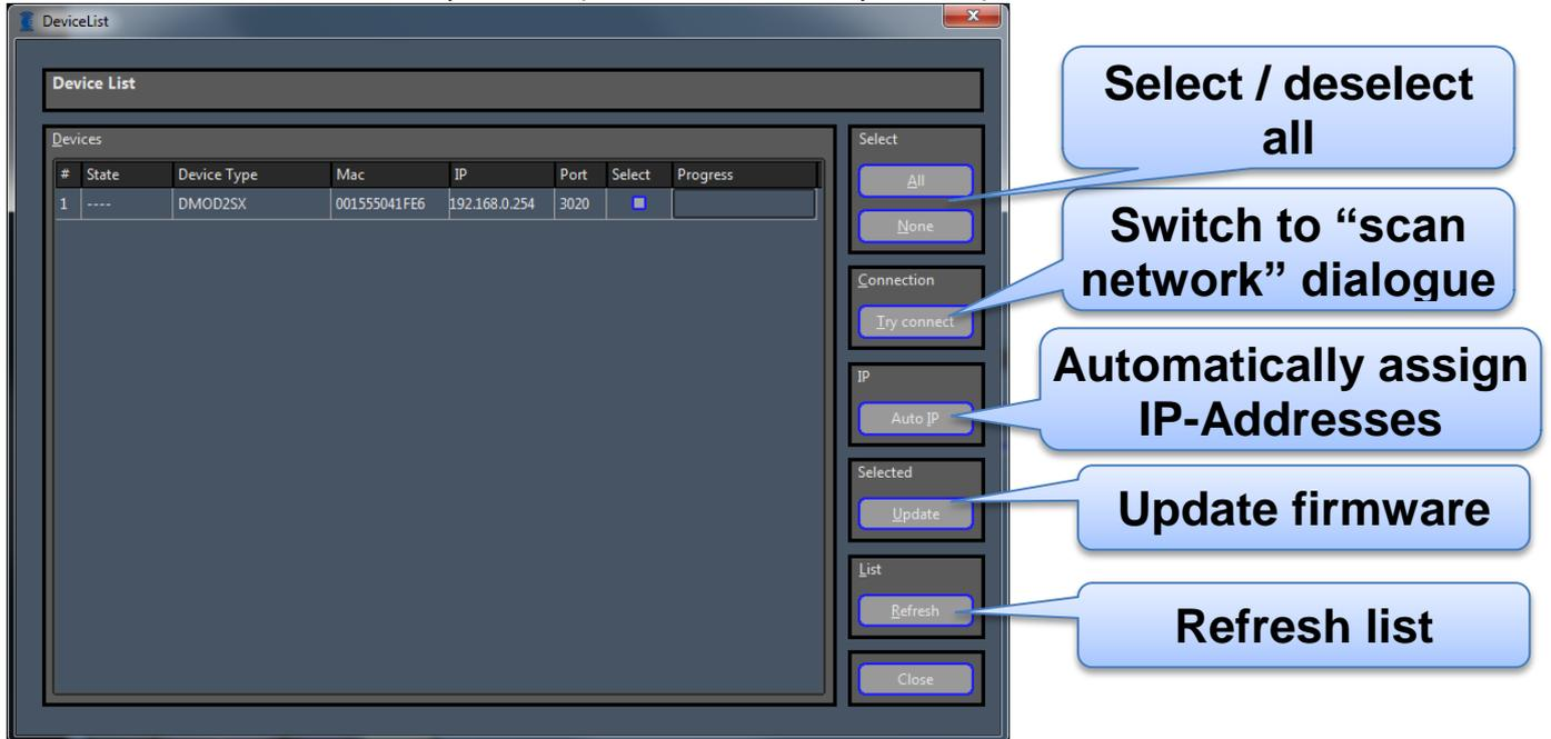
Use the “Auto-IP” button in order to automatically redefine the IP-addresses of connected devices. If several devices are selected successive IP-addresses will be assigned starting from the address specified in the dialogue.
