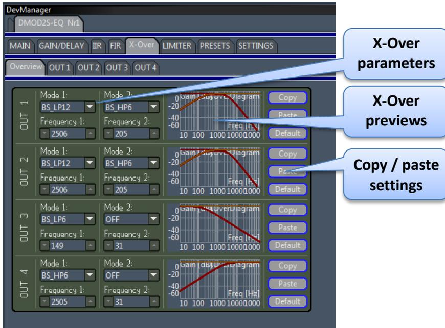
A detailed view for each channel is displayed by choosing the appropriate sub-tab.
