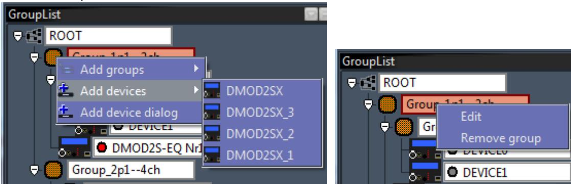
Similarly, to add devices from the network just use the drag-and-drop functionality between the “device list” window and the “group list” window. The information about the group association is automatically stored in the device.
