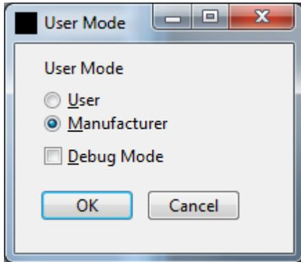
The manufacturer mode is dedicated for the low level adjustment of the audio settings and is password protected.
