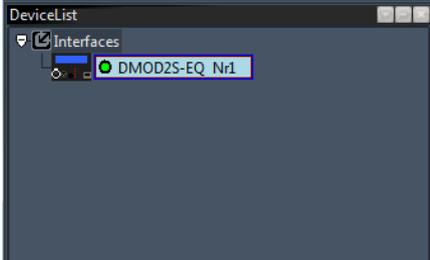
For each device in the network tree a green dot left to the device name indicates that NetControl is currently connected to the device. A red dot indicates that the device is currently not connected. The indicator is yellow while the connection is ongoing.
