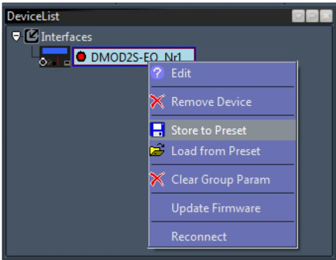
Choosing the “Store to Preset” option from the pop-up menu opens the appropriate file dialogue. In order to retrieve device parameters from a local file the equivalent option “Load from Preset” has to be used. The loaded parameters overwrite the active parametrization data. In order to store them permanently on the device proceed as described above.
