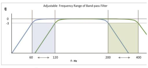
Adjustable Range of Lower Frequency of Band-pass Filter
