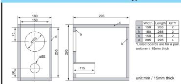
Example of FE126E standard bass reflex type enclosure. Internal volume is 10.5 liters tuned to approximately 61Hz (Fb).
